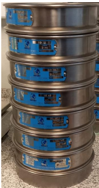
Figure 12 - Sieves with mesh pores ranging from 2 mm (top) to 0.075 mm (second to last), and collection tray (Author's Photography).
