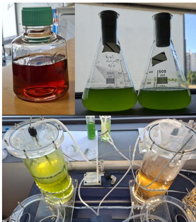
Figure 20 - Filtrated winery-effluent (top-right), Chlorella vulgaris pre-inoculum (top-left) and Column reactors 1 and 2 (bottom). (Author's photography)
