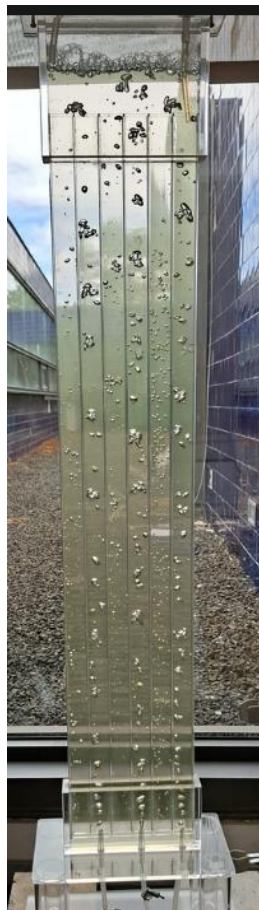
Figure 6 - Flat-panel Photobioreactor. (Author's Photography)
