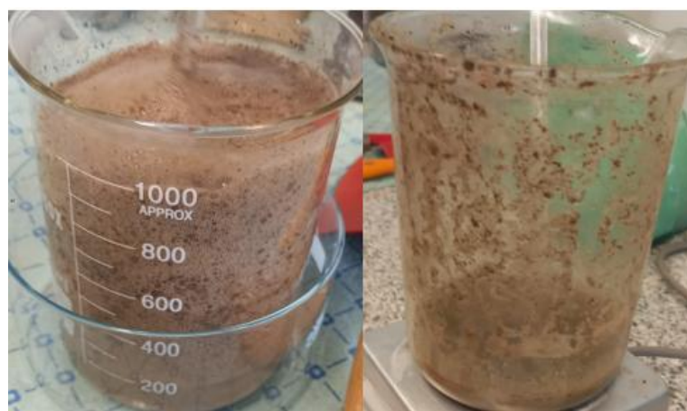
Figure 16 - Soil organic matter reaction with H_2O_2 (left) and soil after reaction with H_2O_2 (right). (Author's Photography)
