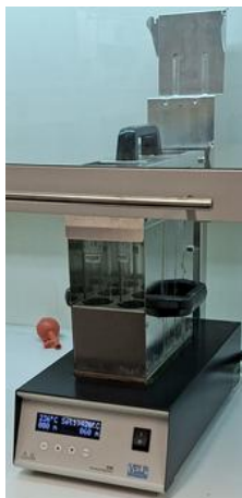
Figure 13 - Velp DK 8 Digestion unit. (Author's Photography)
