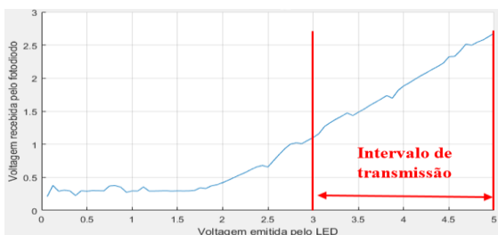
Fig. 13 – Optical power emitted by the LED as a function of the bias voltage
