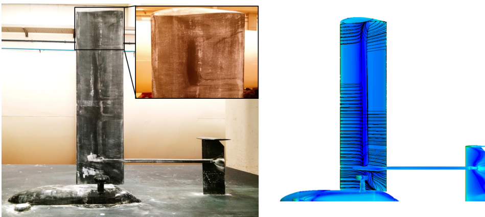
Figure 4.29: Comparison between china-clay flow visualization wind tunnel results ( left ) and skin friction distribution and near surface streamlines from CFD simulations ( right ) over the lower wing surface.
