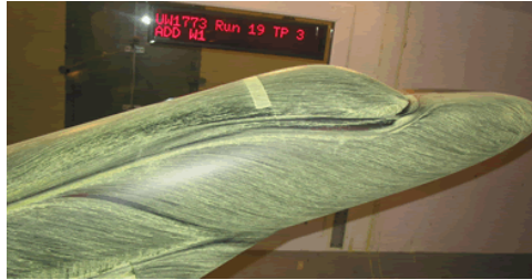
Figure 2.19: China clay flow visualization [University of Washington, College of Engineering, accessed May 23rd, 2016].
