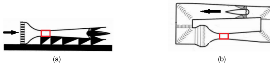
Figure 2.13: (a) Typical layout of an open circuit wind tunnel; (b) Typical layout of a closed circuit wind tunnel [Barlow et al., 1999].
