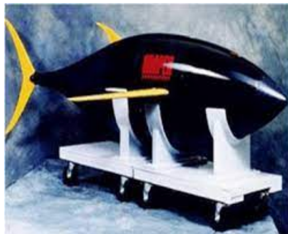
FIGURA 2.15: Vorticity Control Unmanned Undersea Vehicle . Fonte: Anderson e Chhabra (2002)
