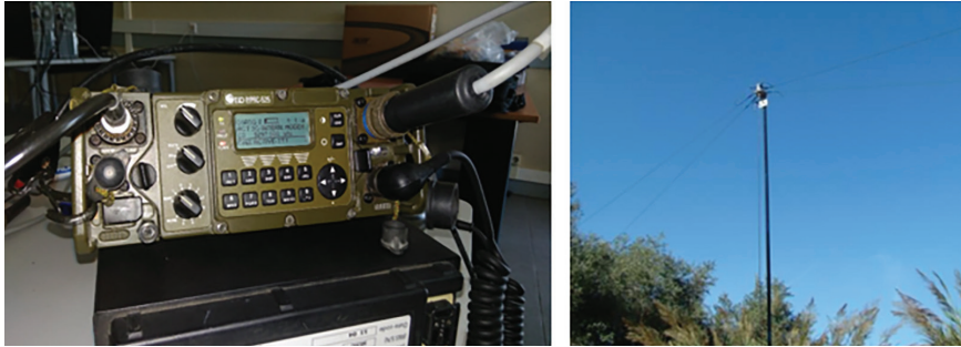
Figure 12 – E/R GRC-525 radio and RF-1936P dipole antenna
