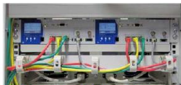
The FCE Controller mounting shelf is 19" wide and 2U high. One mounting shelf accommodates two FCE Controllers side by side.
