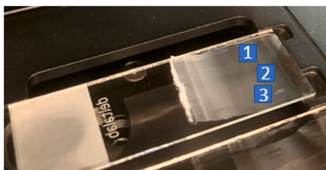
Fig. 5. Glass slide with clobetasol propionate 0.5 mg/g cream exhibiting three distinct representative regions for the automated counting of particles.
