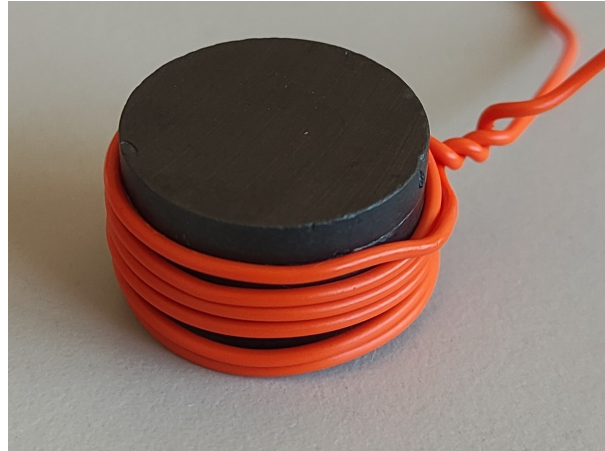
Figure 5.32: Coil with magnets at its center.
