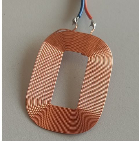
Figure 5.8: Coil taken from Zerone Wireless Power Receiver.
