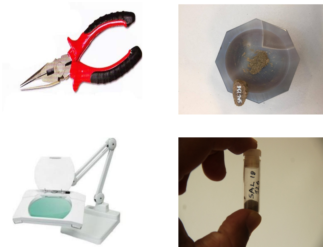
Figure 21: Up Left: Pliers, Up-right: Mortar for making the powder from the samples; Down-left: Desk magnifier lamp; Down-right: Prepared sample for analysis in an airtight tube.
