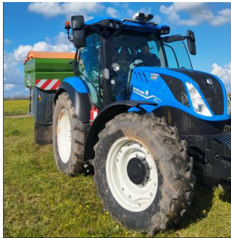
Figura 12 - Trator new holland T5.140 dynamic command™ e distribuidor de adubo Amazone ZA-TS.
