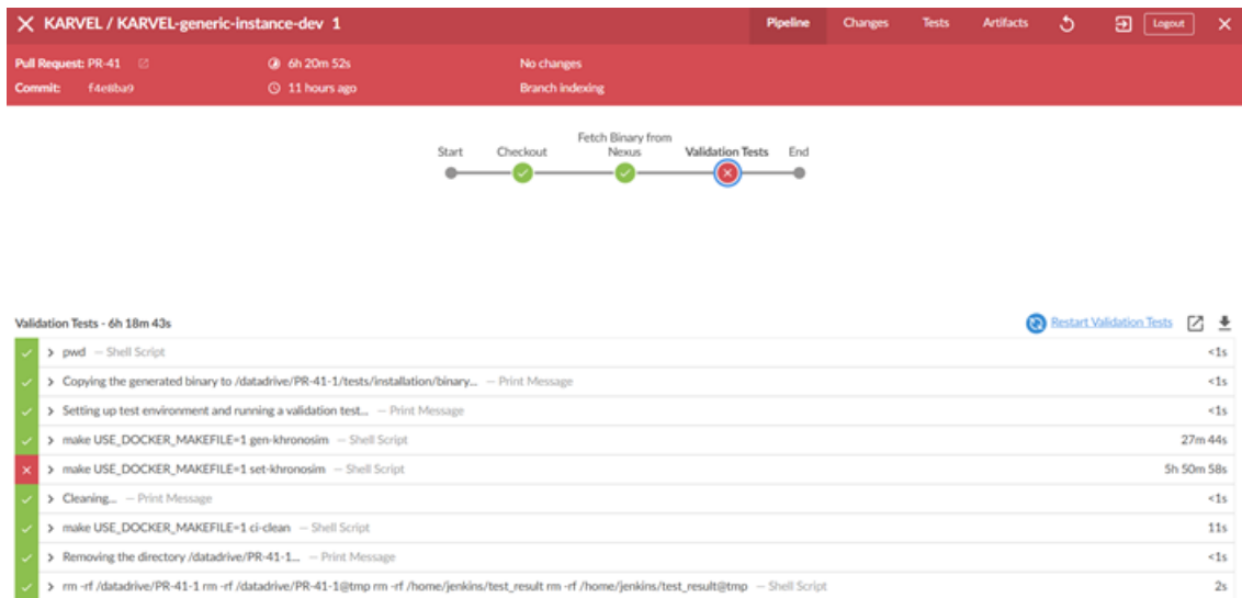
Figure 26 - Jenkins pipeline execution and failure during validation tests
