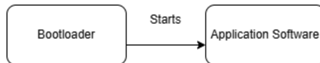
Figure 11 - Bootloader without specific Boot Software
