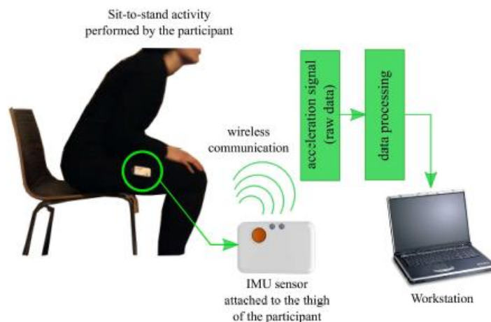
Figure 2.5: IMU sensor attached to the individual's body. (Martinez-Hernandez et al., 2019).
