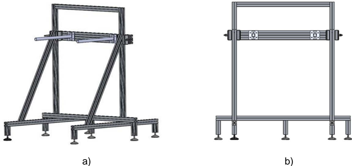
Figure 2.6: Device developed for the assessment of the upper limbs’ assistance. a) Isometric view. b) Front view. (Oliveira, 2021).
