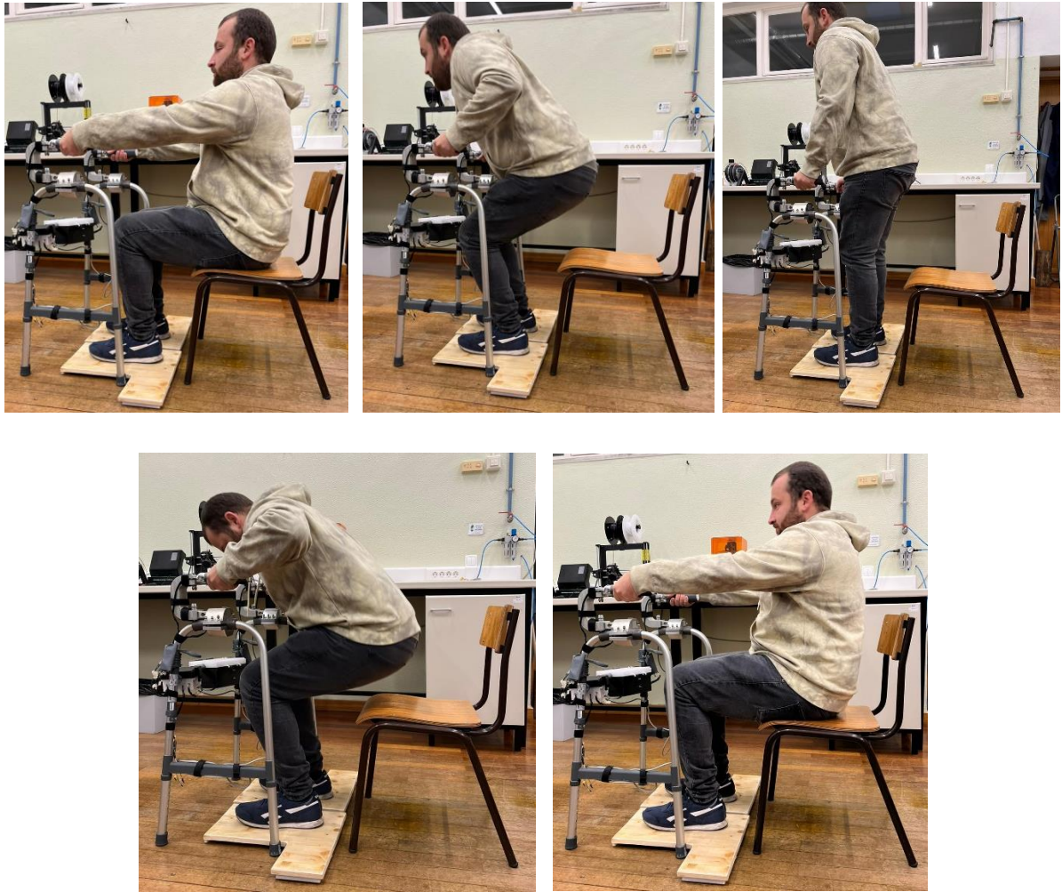
Figure 4.1: Sequence of movement during the STSTS test.
