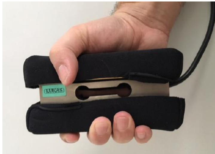
Figure 2.12: Gripping force device with an "S" shape load cell. (Kudrna et al., 2017).
