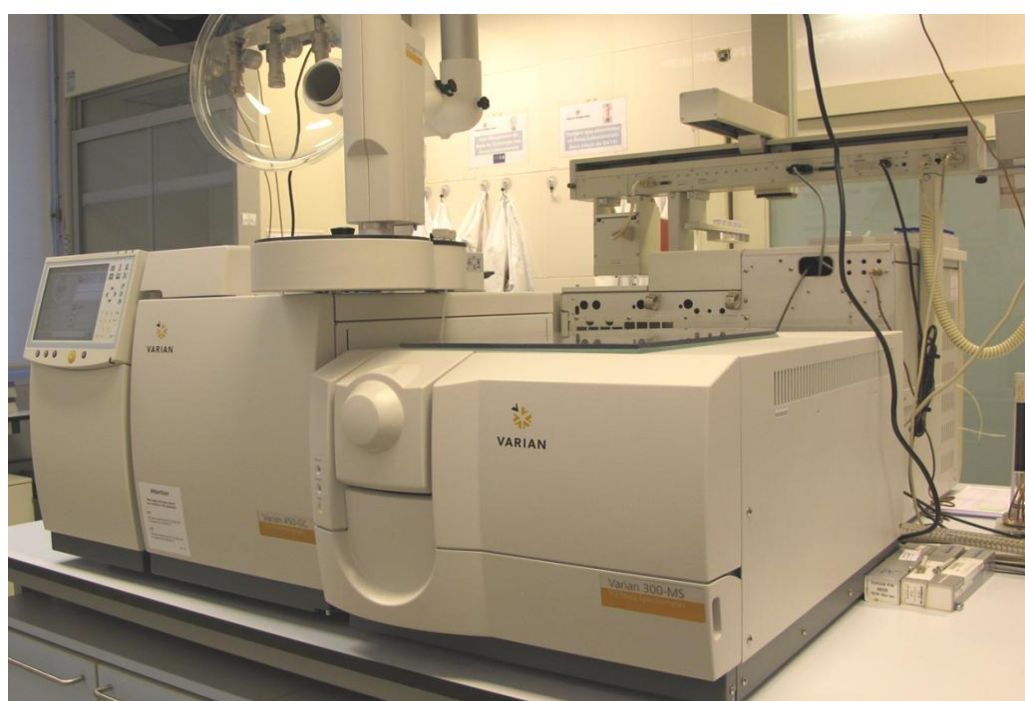
Figure 1 - GC-MS/MS instrument: Bruker GC-450 gas chromatograph coupled to a 300-MS triple quadrupole detector.
