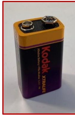
Figure 4.15 Photography of the 9V battery for the power unit of the entire system.
