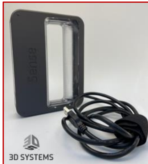
Figure 3.5 3D Scan Equipment "Sense™", used in the project.
