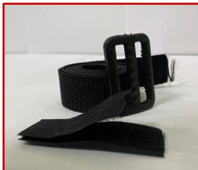
Figure 3.37 Photography of the resistance fabric, slider buckler and velcro tap used in the Resistance Fabric with Velcro mechanism
