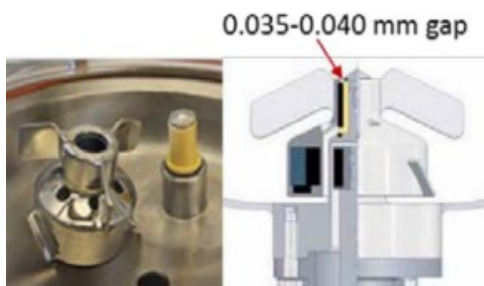
Figure 5. Mavag Mavadrive™ - Gap between the impeller and the drive unit (30)
