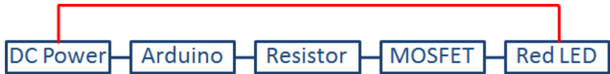
Figure 2. Block diagram for the Red LED test
