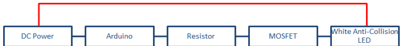
Figure 5. Block diagram for the Anti-Collision White LED test
