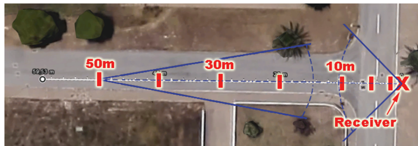
Figure 4.14: Distances and Positions for both Subsystems for transmission's field coverage tests
