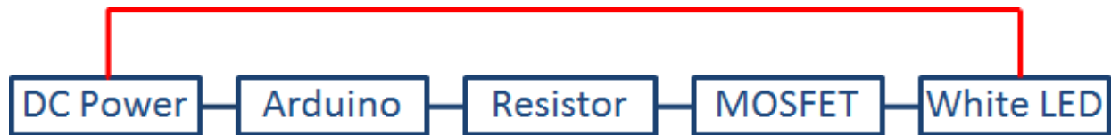
Figure 4. Block diagram for the White LED test
