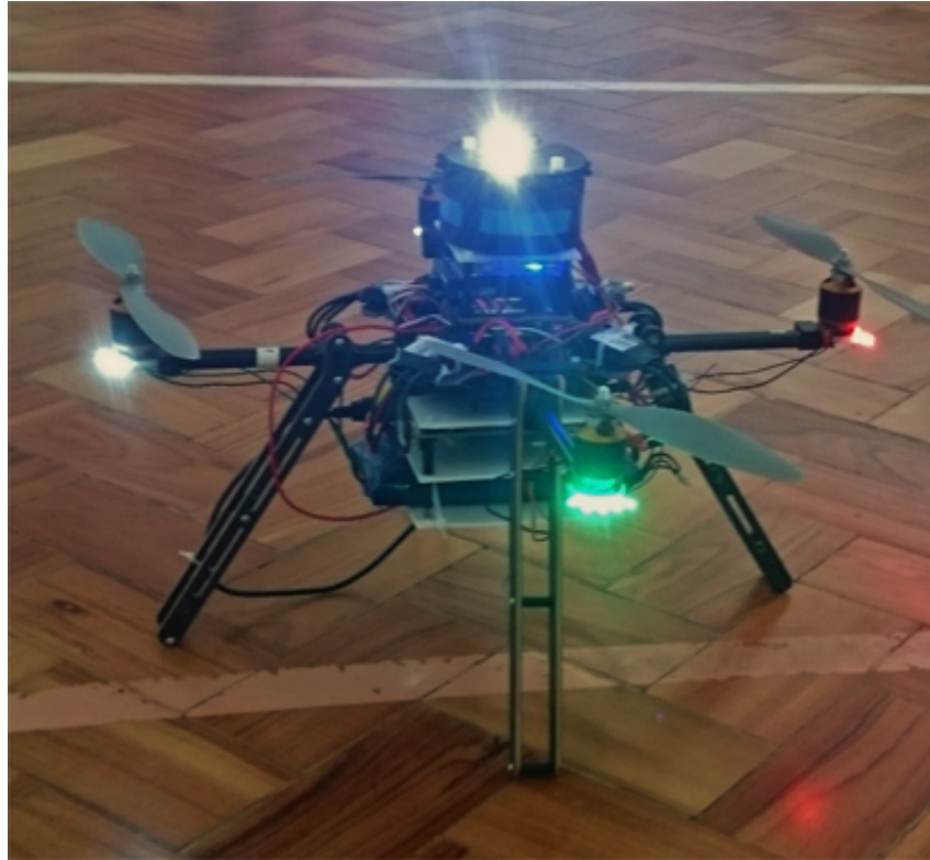
Figure 4.21: IR sense and avoid prototype assembled on quadcopter
