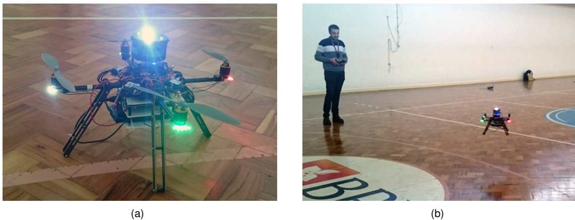
Figure 3.10: Aircraft with visual spectrum solution implemented during flight: (a) ready for take-off; and, (b) mid flight.
