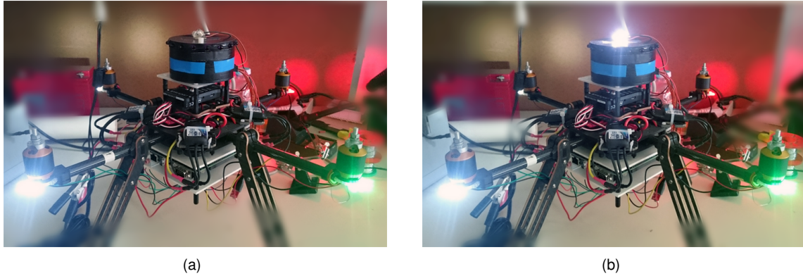
Figure 3.9: Aircraft with visual spectrum solution implemented: (a) with anti-collision light off; and, (b) with anti-collision light on.
