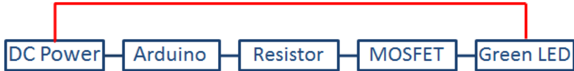
Figure 3. Block diagram for the Green LED test
