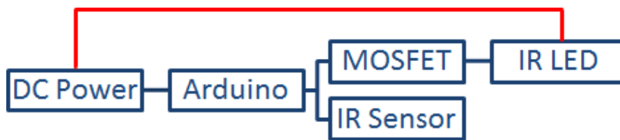
Figure 1. Block diagram of the IR Anti-Collision System
