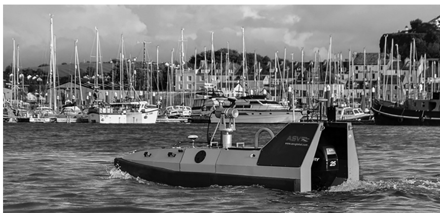
Figure 3 – USV for topo-hydrographic data collection (C-Target 3 ASV)
