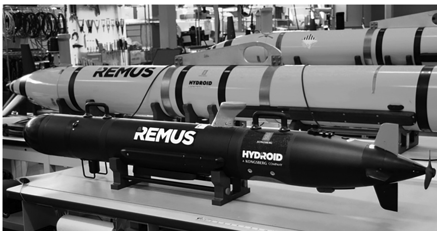
Figure 4 – UUV for hydrographic data collection (Kongsberg's REMUS)
