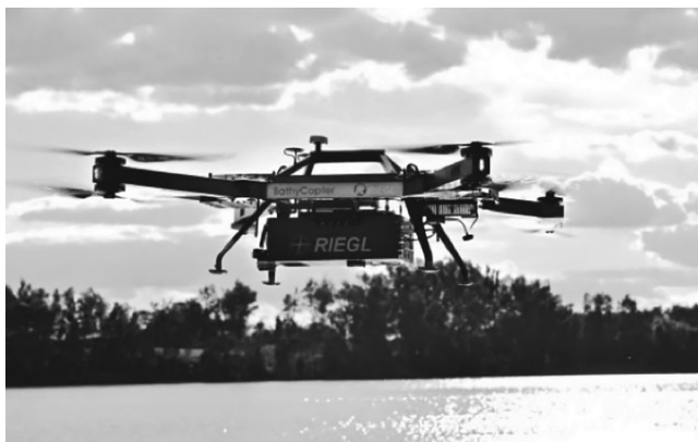
Figure 2 – UAV for topo-hydrographic data collection (RIEGL's BathyCopter)
