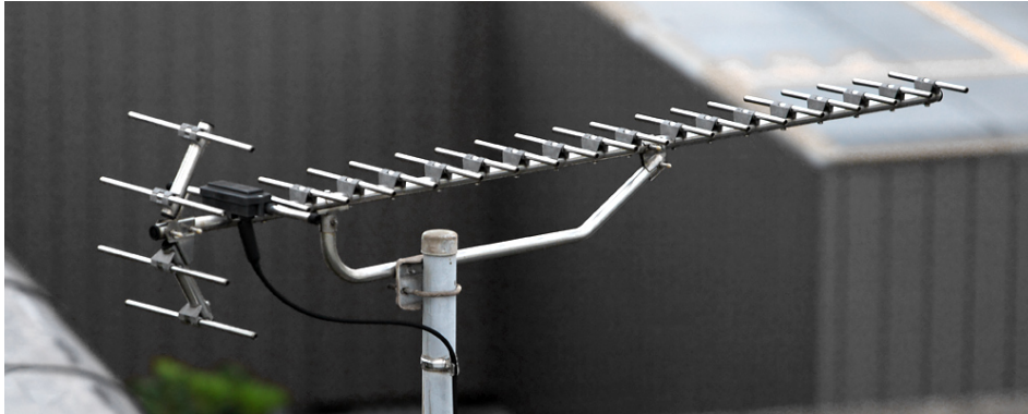
Figure 2.7: Yagi Antenna for Ultrahigh Frequency (UHF) High-Definition Television (HDTV) Reception Source: https://commons.wikimedia.org/wiki/File:UHF_TV_antenna01.JPG
