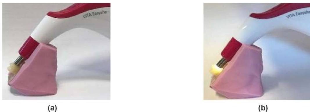
Figure 2. Creation of a pink silicone key and placement of the Easyshade V spectrophotometer to ensure all measurements were consistently taken in the middle third of the buccal surface of the tooth. (a) Position; (b) reading.
