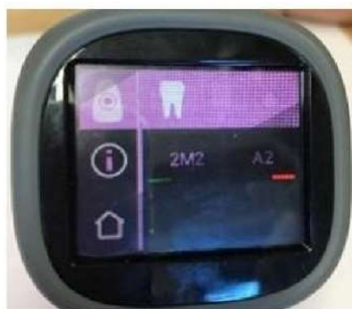
Figure 3. Determination of the tooth color (VITA A2) upon selection on the menu of the equipment and after three consecutive color measurements performed with the Easyshade V spectrophotometer.
