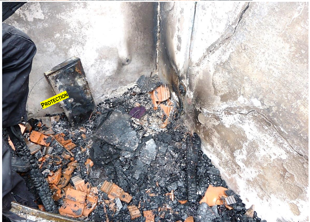
Picture 15 – In the same area the DVD player was recovered, which was disconnected and located on a shelf below the top of the table and showed a similar damage concerning the degree and direction –red arrow.
