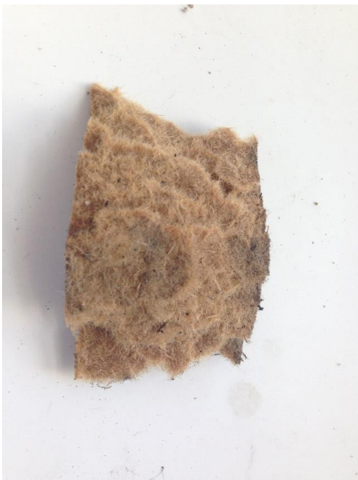
Figure B25: Picture of the skirting board before burning.
