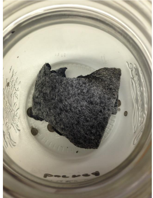
Figure B16: Picture of the carpet underlay after burning.
