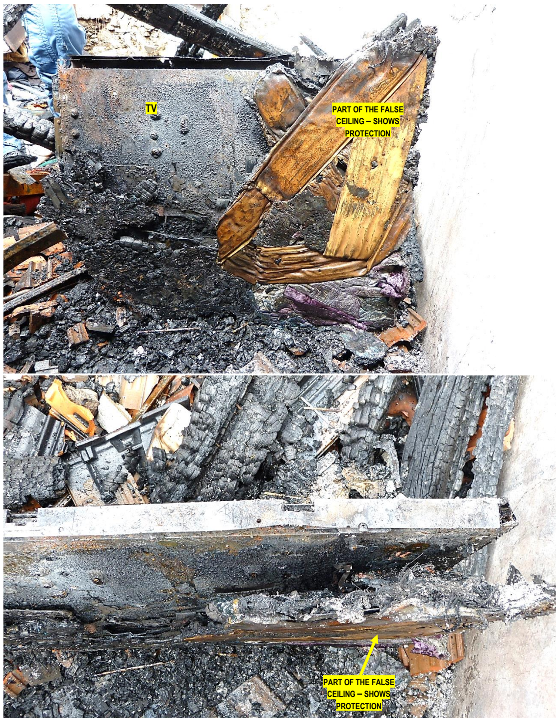
Picture 16 – TV recovered in the debris, which had fallen in front of the table. Underneath the device -due to melting- a section of the false ceiling was identified, which fell on the floor due to the heat received by the spread of the fire before the fall of the TV.
