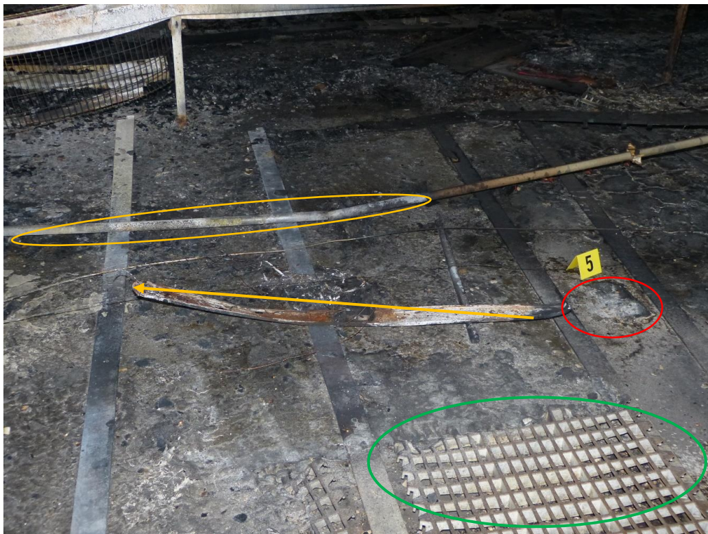
Picture 11 - Tag #5 – residues of second detoxification bloc (red circle) and potential area for point of origin; signs of high exposition levels can be observed on the metal bars (orange ellipse), increasing from the right to the left of the picture (south to north) with signs of oxidation (orange arrow); presence of part of the PVC-roof (green circle) indicates that the fire was not travelling towards that direction, since it otherwise would have destroyed it completely, but it was affected by radiant heat of being in close proximity of the fire.
