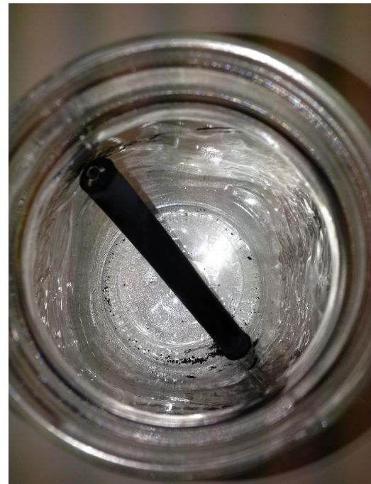
Figure B34: Picture of the electric cable with three conductors after burning.
