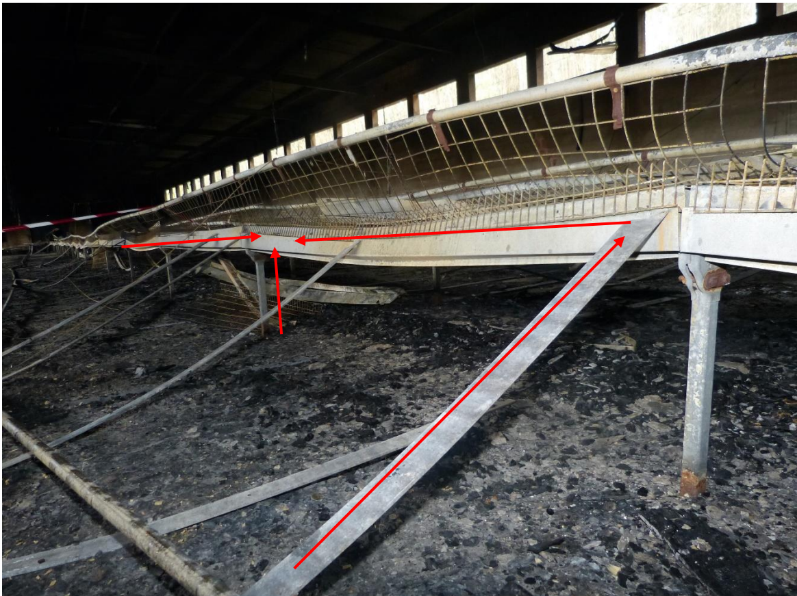
Picture 19 - View of metal bars on left side of pavilion from potential seat of fire south to north – decreasing levels of oxidation and damage from south to north and from east to west, red arrows indicate the increasing level of damage pointing towards one area of origin.
