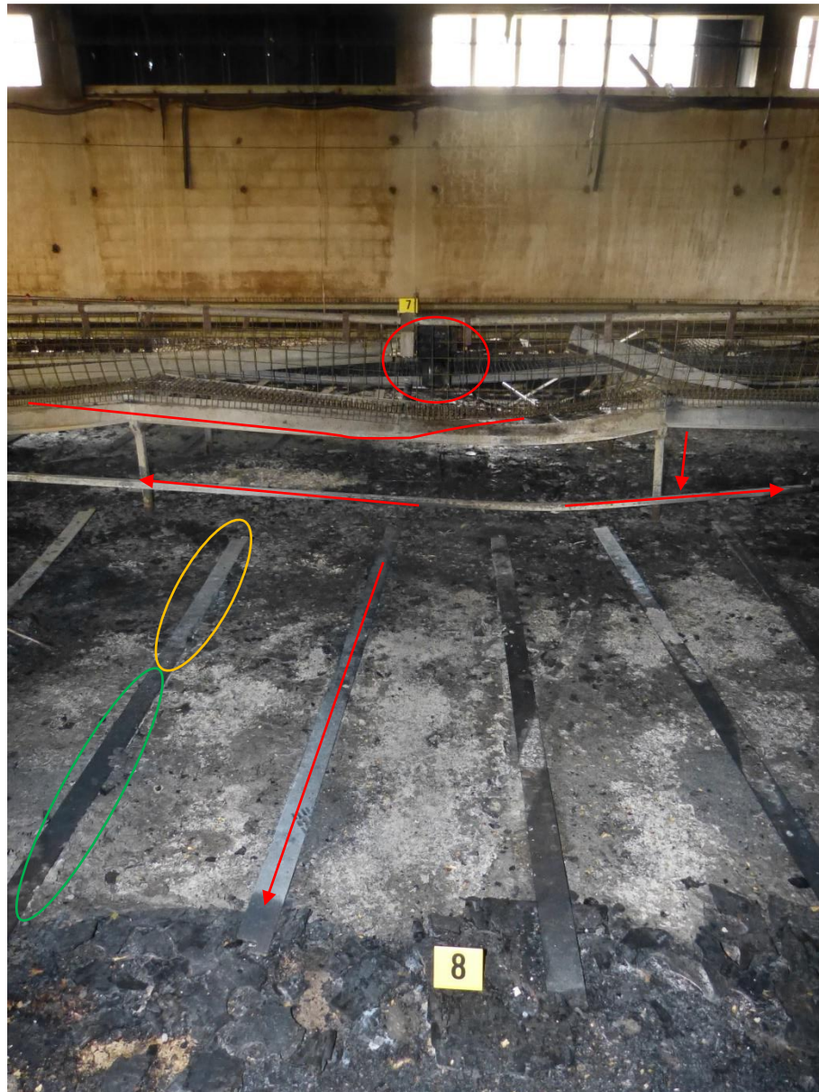
Picture 33 - Tags #7 and #8, view from west (bottom) to east (top) – second potential seat of fire; red arrows indicate the probable direction of propagation of the fire, due to increasing damage levels in a concentric way towards one point (red circle), highest point of deformation of the metal bars, also signs of prolonged exposition to high temperatures, exposition signs are strong; metal bars on the floor show decreasing damage signs from top (east) to bottom (west).
