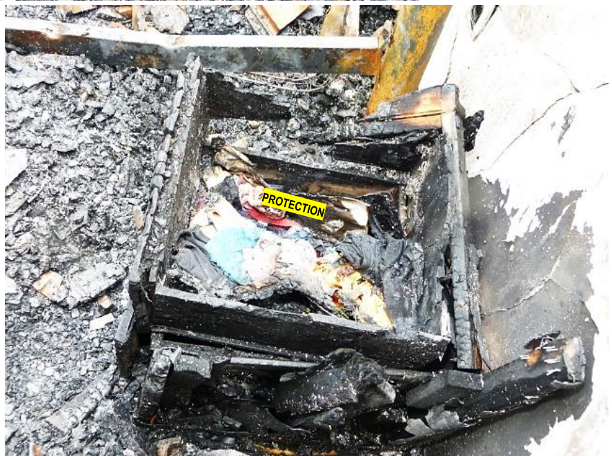
Picture 22 – Overview of the area with higher degree of damage - the high damage to the chair results from the heat received directly by the emissions of the starting point of the fire, which led to the subsequent light-up of the chair .On the side of the table exposed to the chair and in its interior some areas of protection are observed, determining the development of combustion from an higher area, at a level around the top of the table.
