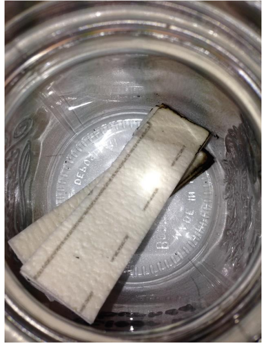
Figure B12: Picture of the vinyl flooring kitchen-use after burning.
