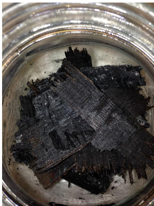
Figure B2: Picture of the plywood flooring after burning.
