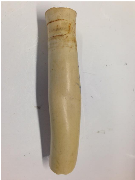
Figure B29: Picture of the gas pipe before burning.
