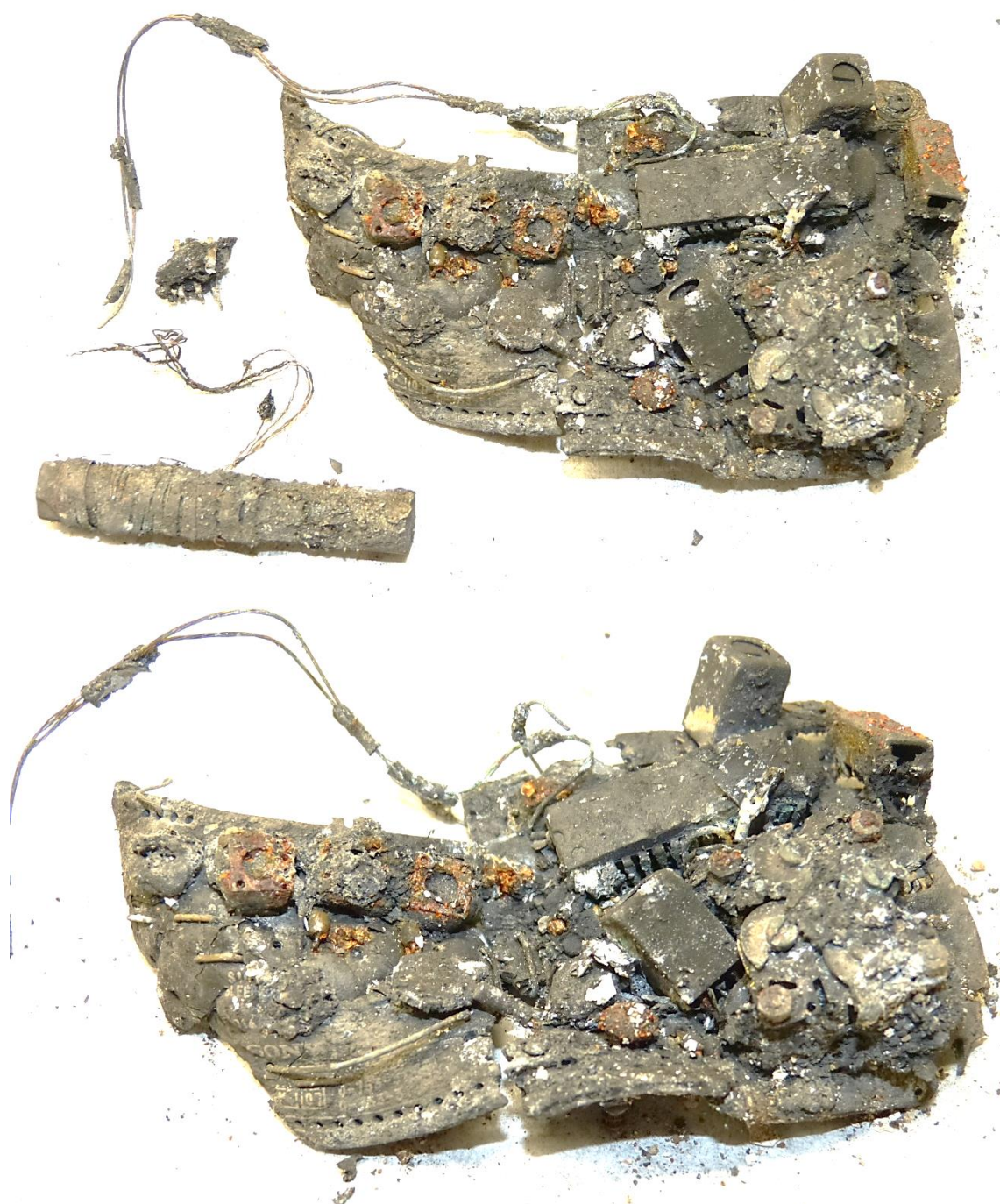
Picture 24 – Detailed view of the remains of the electrical components belonging to the alarm clock after cleaning of the fire debris. Homogeneous damages can be observed, which result from the reception of an external heat source.
