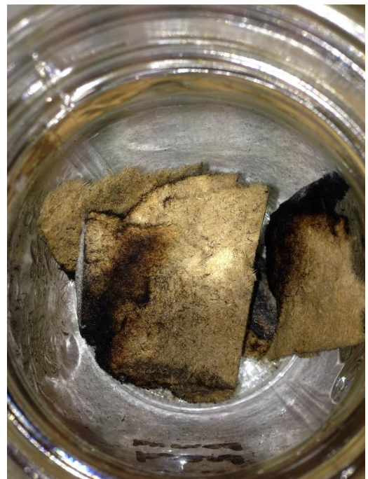
Figure B26: Picture of the skirting board after burning.
