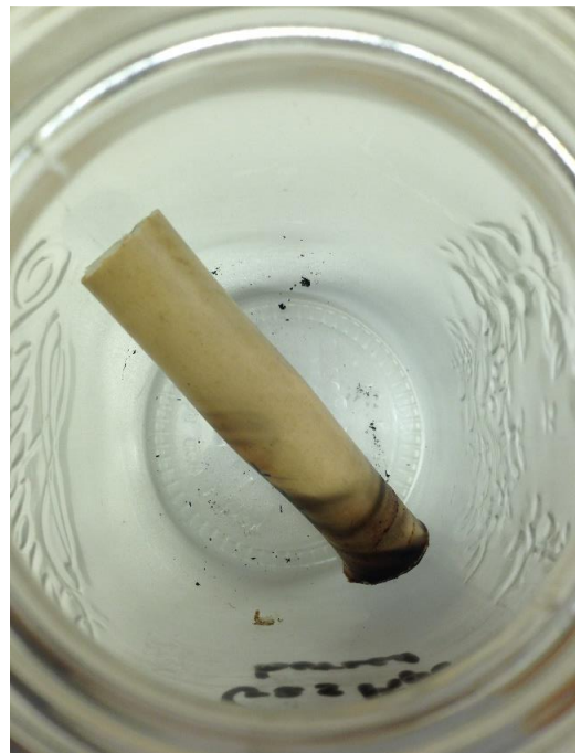
Figure B30: Picture of the gas pipe after burning.
