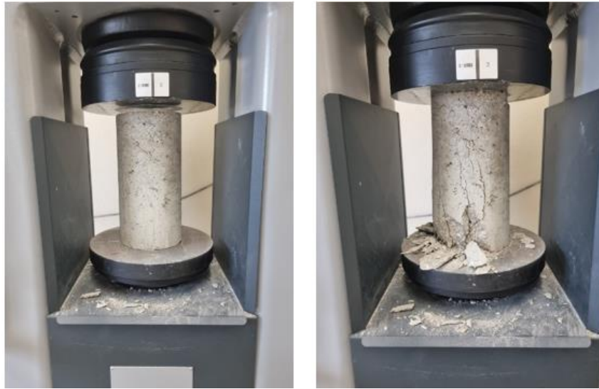
Figure 4.11: Initial placement, and the final state of the concrete specimen after failure.
