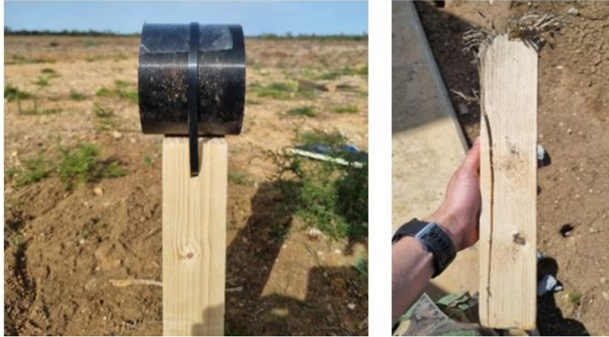
Figure 4.15: EFP attached to the disposable support as well as the support after the detonation occurred.
