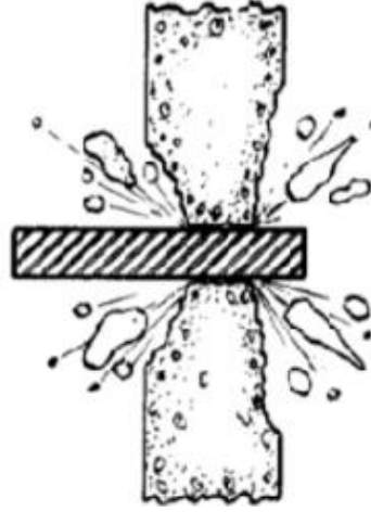
Figure 2.7: Perforation of concrete caused by a projectile [28].
