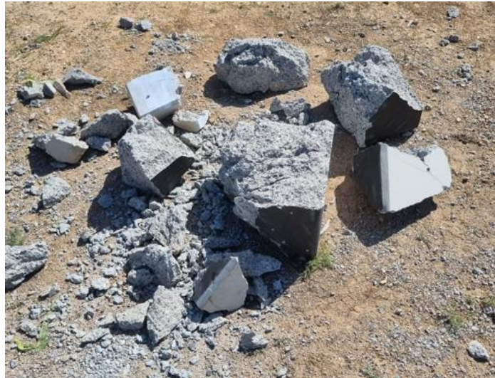
Figure 4.25: Block 4 after the impact.
