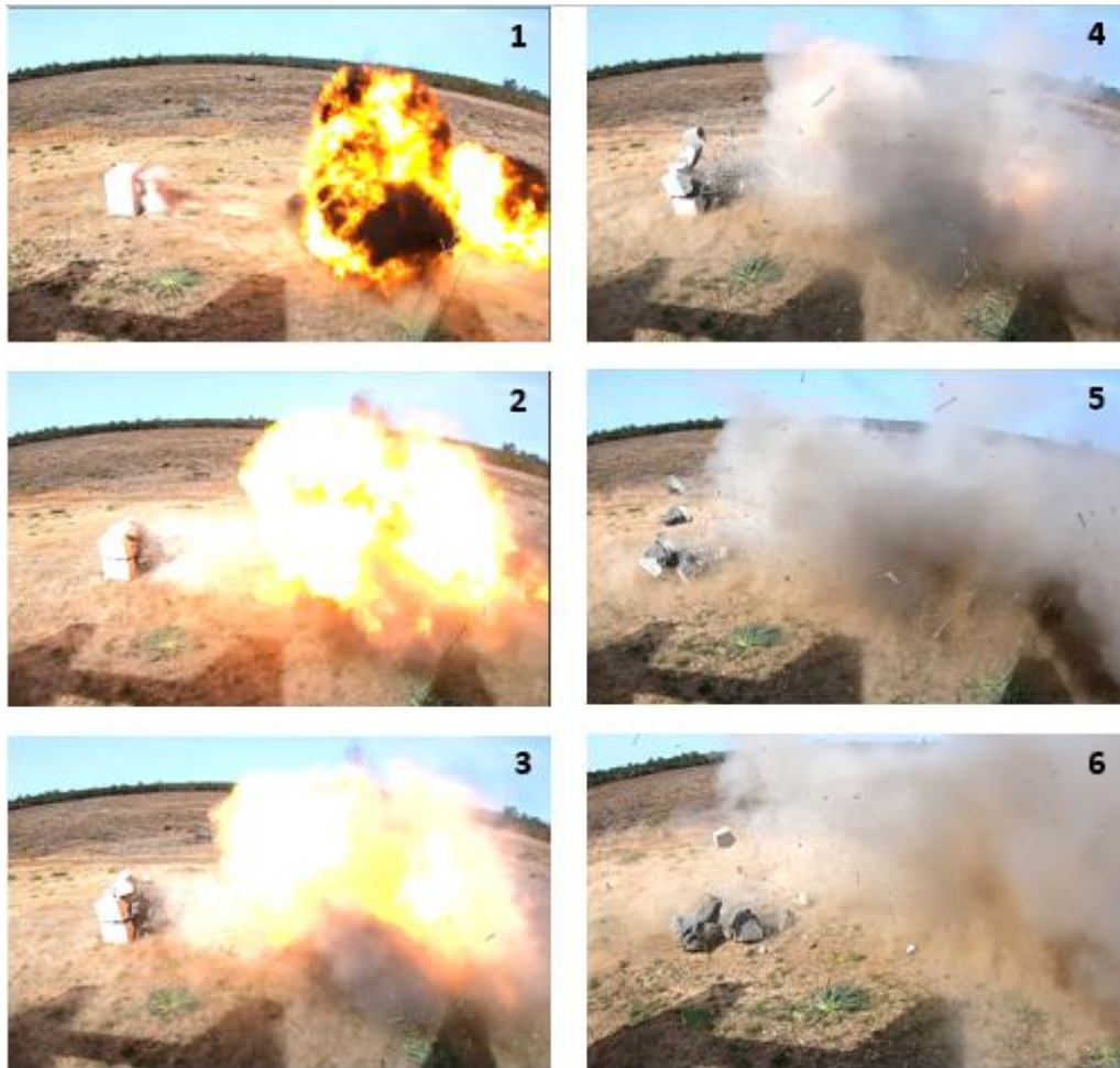
Figure 4.27: Sequence of frames of EFP impacting the concrete block.
