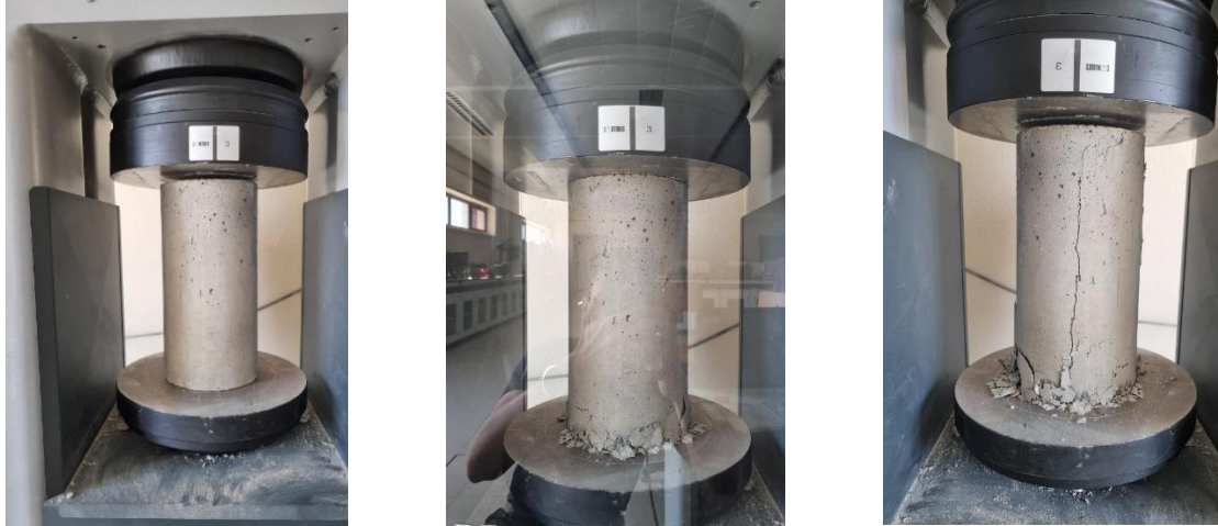
Figure 4.9: Different stages of the concrete cylinder, including its placement, the halfway point of the test, and the result of the concrete.
