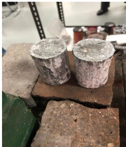
Figure 3.7 - Samples after the hot compression.
