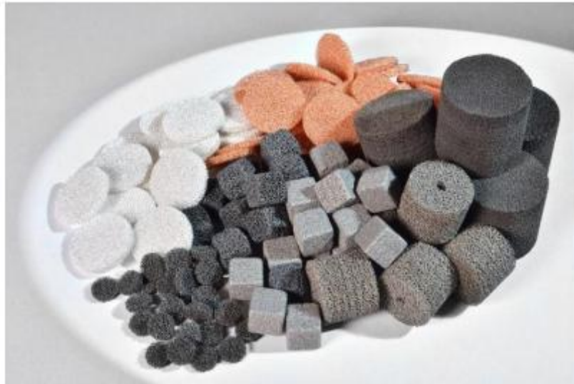
Figure 2.22 - Different pure metallic and alloyed foam pellets for catalysis in packed bed reactor vessels [67].
