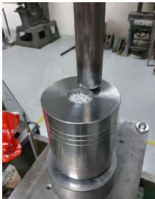
Figure 3.2 - Mould used for the preparation of the samples.
