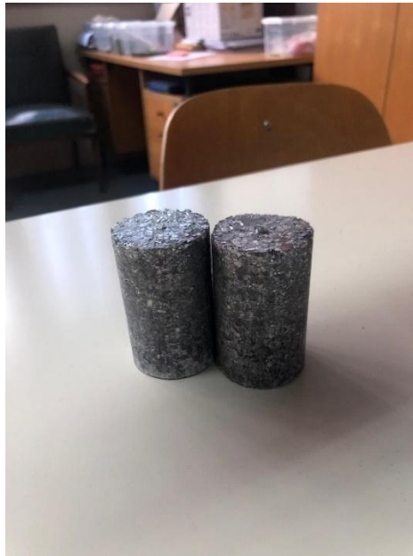
Figure 3.5 - Example of two samples after the cold compression.
