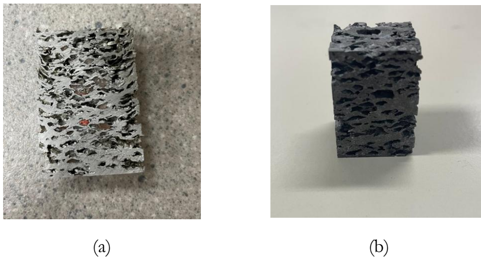
Figure 3.9 - (a): Sample after the cut; (b): Sample after boiling in water again.
