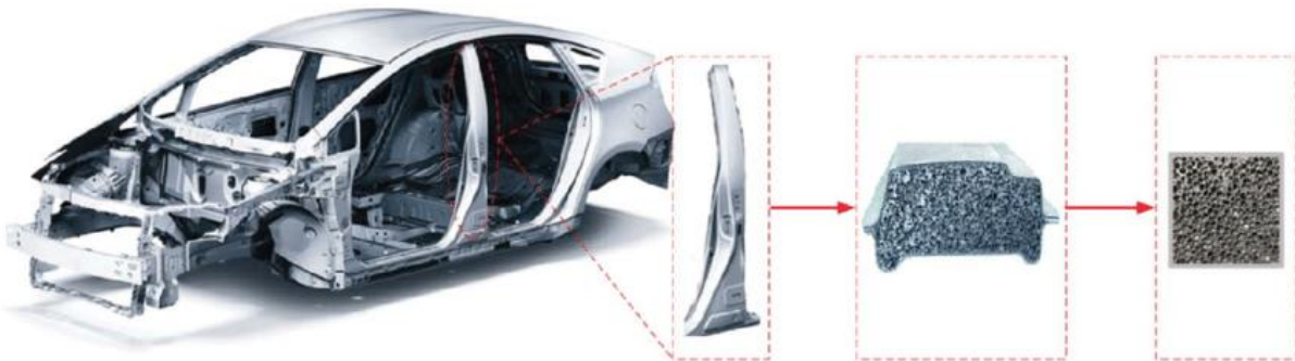
Figure 2.21 - The typical foam-filled tubular thin-walled structure in a vehicle [66].
