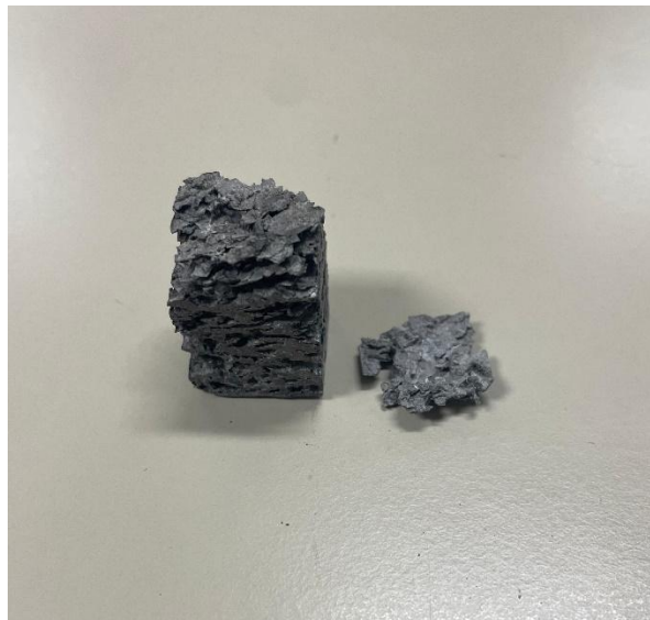
Figure 3.15 - Sample 3 showing localized fracture and loss of material.
