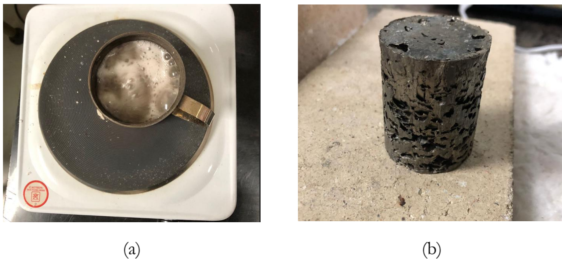
Figure 3.8 - Boiling water process: (a)- Boiling the sample; (b)- After boiling.
