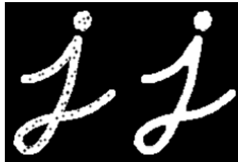
FIGURA 2.7: Closing. Retirado de OpenCV Development Team (2025).
