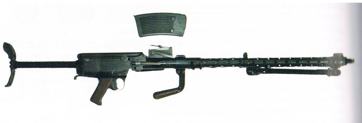
**Figura 0-18 – ML Dryse 7,92mm**
