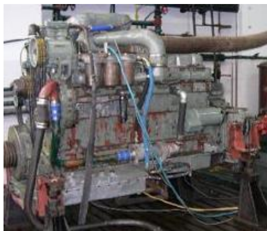
Figura 28 - Motor Diesel Rolls-Royce do locotrator Sentinel, [9].
