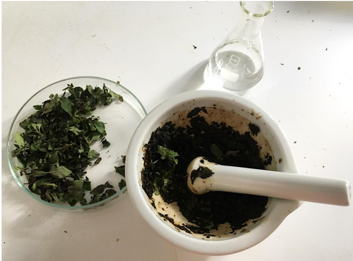
Figure 5 Smashing Origanum vulgare leaves in a porcelain mortar with 100 mL distilled water
